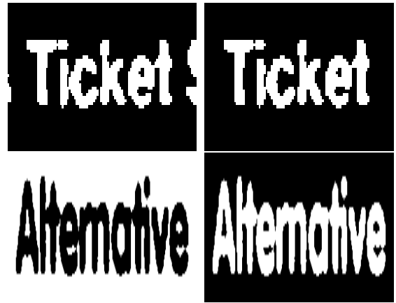
Fig. 2. Binarization of two sample word images using Otsu's method. In the second example, the binarized image is inverted, since we require polarity of text to be brighter than the background.
