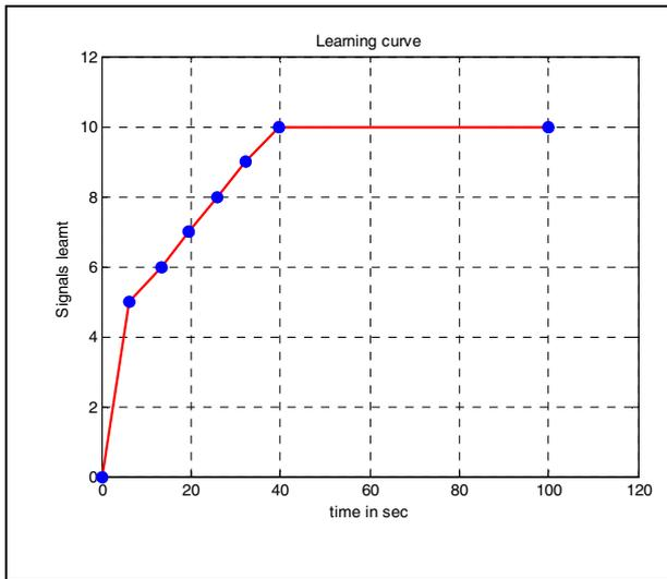
Fig. 3. The curve shows how the correlation structure is learnt by the system. The blue circles indicate the points at which a new signal is added.
