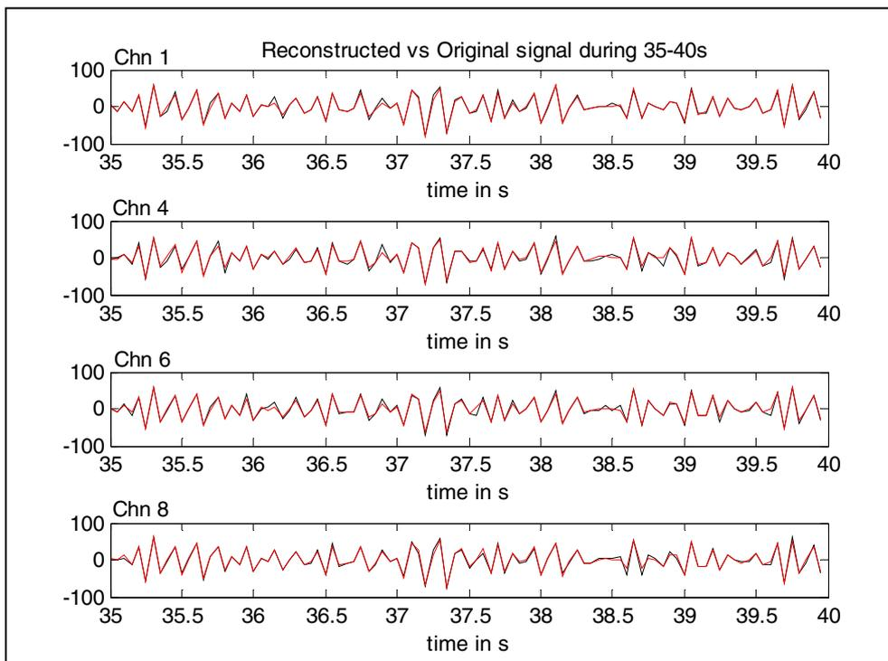
Fig. 2. Reconstructed signal (shown in red color) is plotted against the original signal for four channels, 1, 4, 6 and 8 during the interval 35-40sec. The corresponding PSNR values in dB are: 25.6, 23.3, 22.6 and 24.0.
